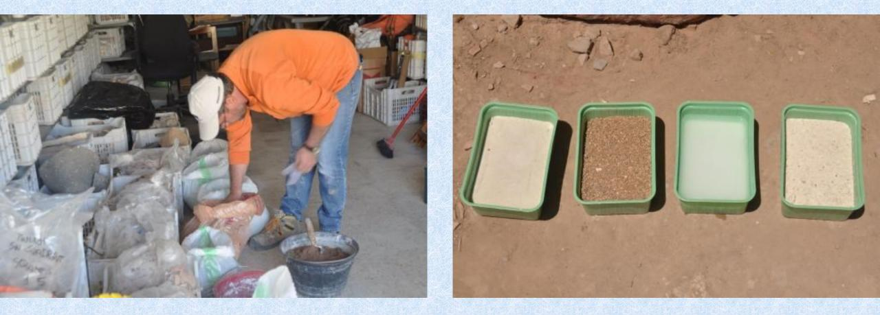
Base-Lime Mortar Test with different Lime (Hydrated and Hydraulic) and different aggregates
