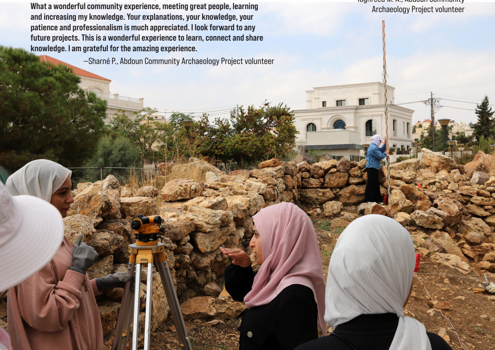
Trained volunteers surveying with an optical level for the Abdoun Community Archaeology Project.
